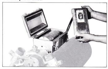
This attachment is designed to prevent water from getting into the motor and causing short circuits.
