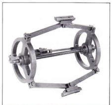
Prevents deformation of large pipes during cutting.
